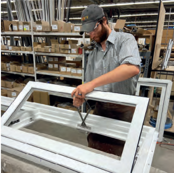
Zach Carr builds a casement window with hardware from Roto Frank of America.
